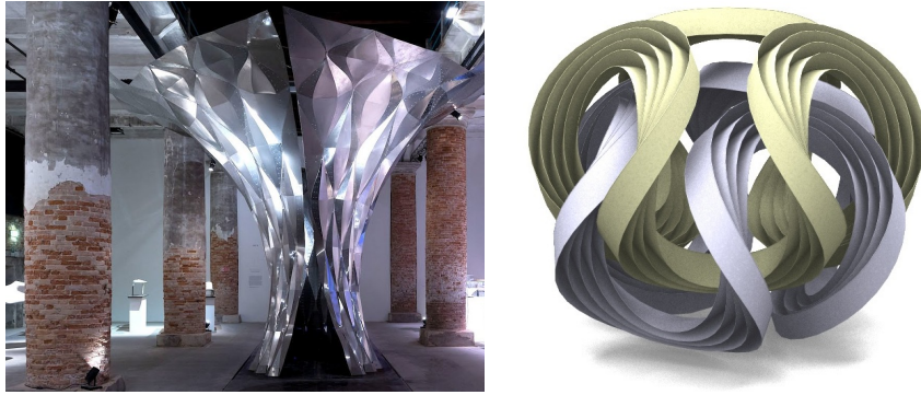
FIGURE 2. Curved-Crease Sculptures. Left: Arum installation, 2012 Venice biennale, by Zaha Hadid architects and Robofold. Its form is defined by sheet metal folded along curved creases. Right: This virtual model of annuli folded along concentric rings by (Tang et al., 2016) is motivated by actual paper objects, cf. (Demaine and Demaine, 2012).
