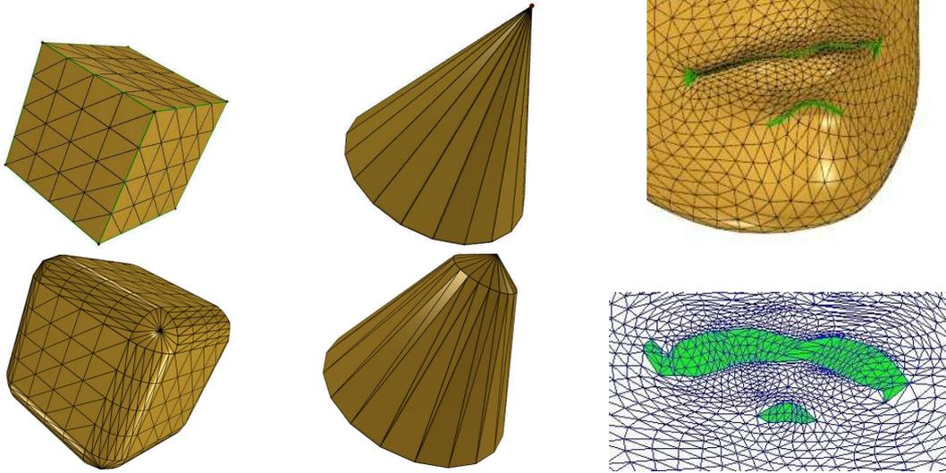
Fig. 2. The blow-up phenomenon at sharp edges and corners: Top: original mesh in  $\mathbb{R}^3$ . Bottom left and center: projection of the corresponding mesh in  $\mathbb{R}^6$ . Bottom right: Parametrization of the corresponding mesh in  $\mathbb{R}^6$ .
