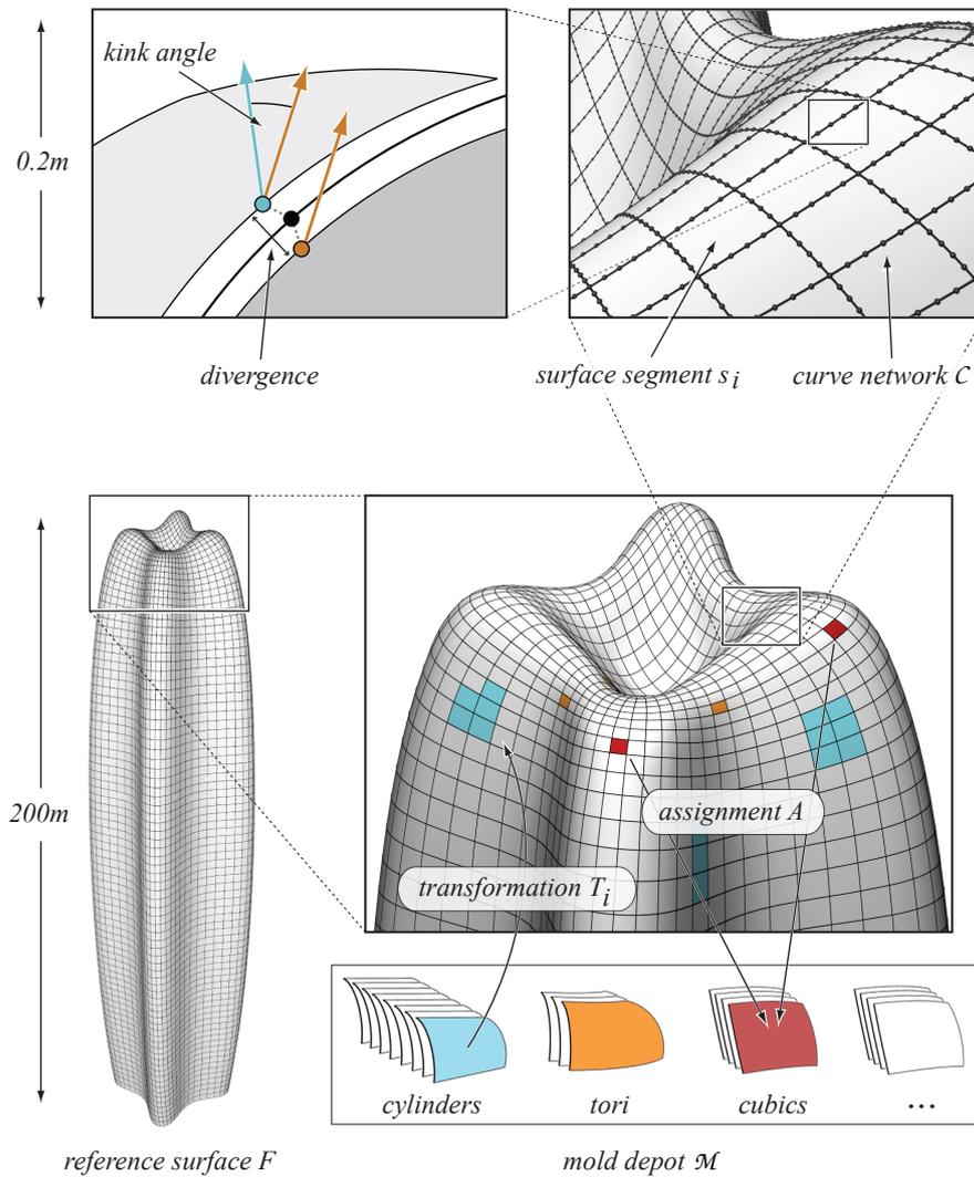
**Figure 5:** Terminology and variables used in the paneling algorithm. The reference surface  $F$  and the initial curve network  $C$  are given as part of the design specification. The optimization solves for the mold depot  $\mathcal{M}$ , the panel-mold assignment function  $A$ , the shape parameters of the molds, the alignment transformations  $T_i$ , and the curve network's normal displacement. Figure taken from [Eigensatz et al. 2010].
