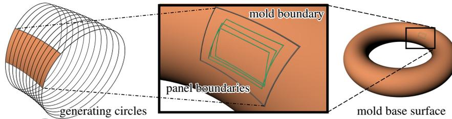
**Figure 6:** Example of mold reuse. Panel boundary curves are in general not congruent. However, several panels may be closely grouped together on the same mold base surface. In that case the same mold or machine configuration, which embraces all affected panels, may be used to manufacture the panels. This figure further illustrates how the congruent profiles of a rotational or translational surface, in this case the circles generating a torus, can be exploited for mold fabrication.
