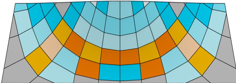
**Figure 8:** Illustration of the mold depot and the cost model by means of the example shown in Figure 3(e). The colors of panels are saturated according to mold reuse. Figure 4 lists the glass cost ratios used for this example.
