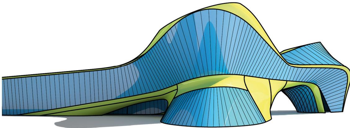
**Figure 5. Large parts of the facade of the Cagliari Contemporary Arts Center by Zaha Hadid Architects have been rationalized with ruled surfaces.**
