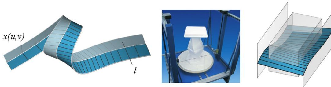
**Figure 1. A ruled surface is formed by a continuous family of straight line segments  $l$ . A ruled surface strip model is composed of several ruled surface patches, glued together in a smooth way (left). Many production processes are based on ruled surfaces, e.g. heated wire cutting (center and right), where the heated wire moves on a ruled surface. Our goal is to approximate free-form shapes by ruled surfaces to take advantage of cost-effective fabrication options.**
