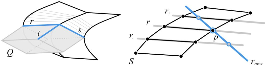
**Figure 8. Tangent continuity of a ruled surface strip model implies vanishing volume of the parallelepiped  $Q$  spanned by the ruling directions  $r$  and  $s$  and the common boundary curve tangent  $t$  (left). The next strip's ruling in point  $p$  of a discrete curvature continuous strip model  $S$  is obtained as common intersection line  $r_{new}$  of  $r_-$ ,  $r$  and  $r_+$  (right).**
