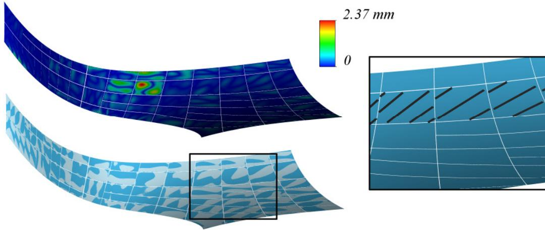
**Figure 6. (Top, left) For a 54 m<sup>2</sup> facade detail of SOHO Galaxy by Zaha Hadid Architects, the maximal deviation of the ruled surface approximation is below 2.4 millimeters. (Bottom, left) shows both reference (grey) and approximated ruled panels (blue). The zoom-out (right) illustrates the ruling direction for some panels.**
