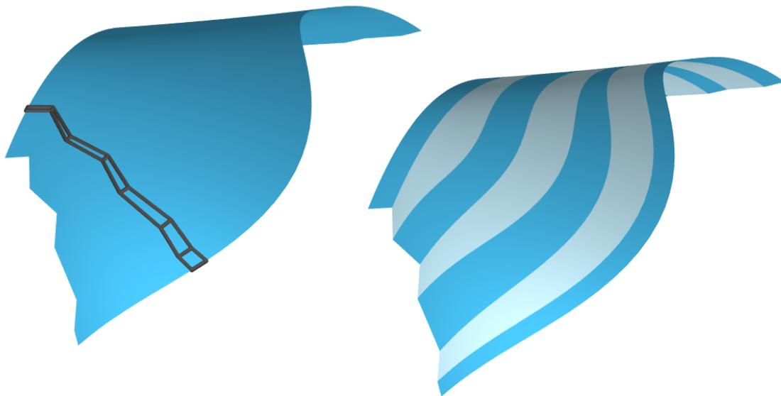
**Figure 10.** A curvature continuous surface formed by a sequence of ruled surface strips has been generated in a parametric model which starts with a single strip and automatically adds further strips so that curvature continuity is achieved. The shape is controlled by the first strip and the width function for the other strips. The left-hand side shows the zigzag pattern of rulings, which is necessary to obtain curvature continuity.
