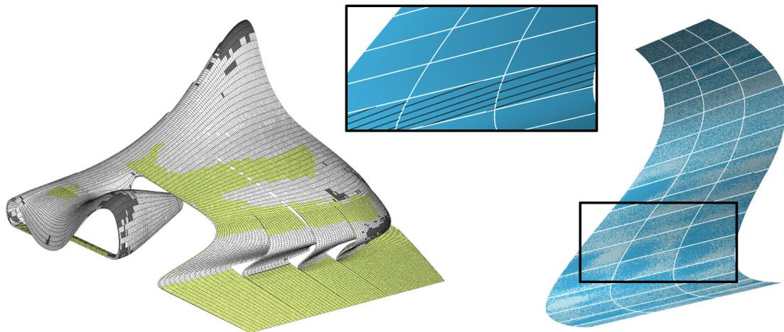
**Figure 7.** The panels of the Heydar Aliyev Cultural Centre facade by Zaha Hadid Architects are classified for planar (green), ruled (light grey) or general double curved (dark grey) rationalization (left). The ruled surface approximations of a subset of 51 panels are shown on the right, with some ruling directions visualized in a zoom-out (center).
