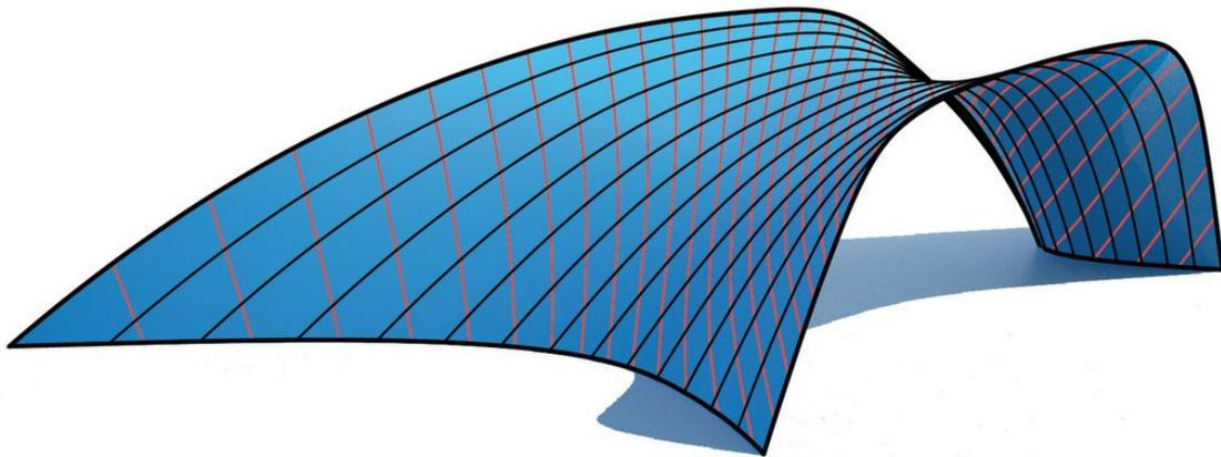
**Figure 9.** This saddle surface, a detail from the facade of the Cagliari Contemporary Arts Center, has been rationalized with 14 ruled surface strips. The strips have been simultaneously optimized towards a smooth overall surface under the constraint that the transition curves lie in user-specified vertical and coaxial planes.
