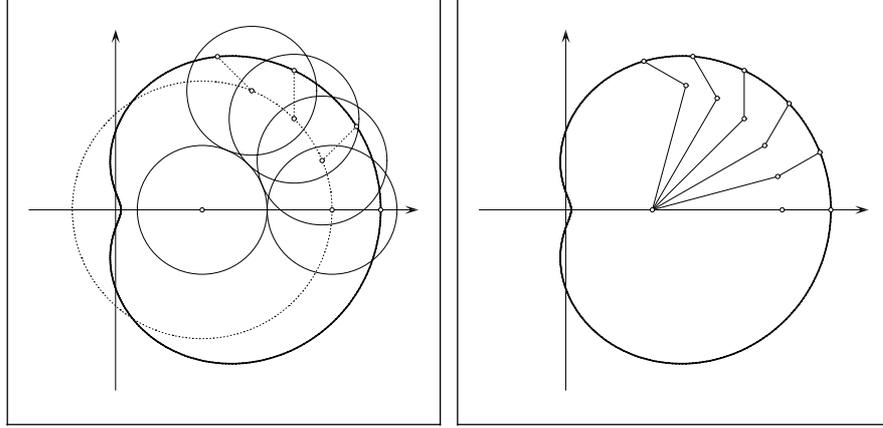
Figure 9. Generation of the limaçon of Pascal as a trochoid by: rolling motion of a circle of radius  $R$  on a fixed circle of radius  $R$  (left), and a two-bar linkage with links of length  $2R$  and  $R^2$  and angular velocities in the ratio 1:2 (right).
