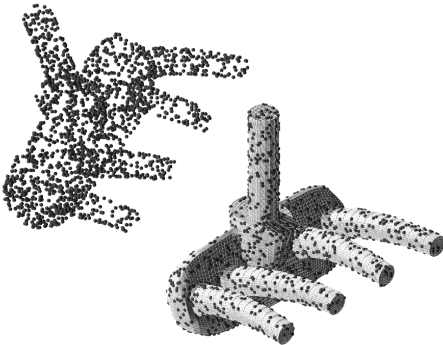
FIG. 4 Registration of a point cloud to a surface. Initial position (point cloud displaced to the upper left), and final position (point cloud in correct alignment with surface model).
