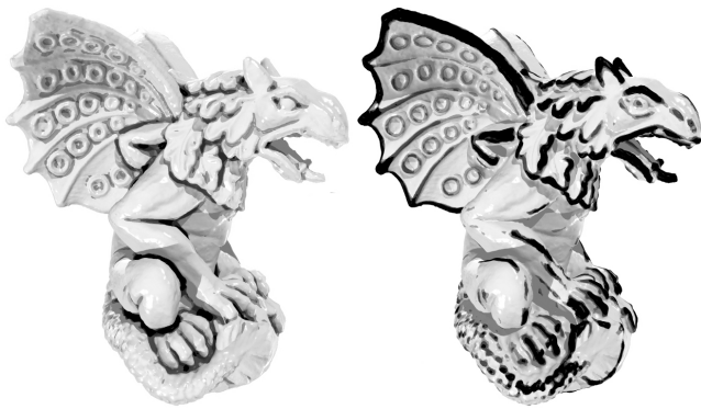
Figure 9: Feature extraction on multiple scales according to [Yang et al. 2006]. Integral invariants for several different kernel radii are used to identify features. Darker regions are classified as features on all scales, lighter shaded regions correspond to features extracted at only one or two scales. At left: ravines; at right: ridges. The integral invariants used for this figure are I_r(x_i x_j) ( i, j = 1, 2, 3 ), whose properties are not discussed in the present paper.
