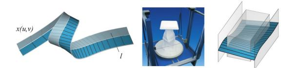
Figure 1. A ruled surface is formed by a continuous family of straight line segments *l*. A ruled surface strip model is composed of several ruled surface patches, glued together in a smooth way (left). Many production processes are based on ruled surfaces, e.g. heated wire cutting (center and right), where the heated wire moves on a ruled surface. Our goal is to approximate free-form shapes by ruled surfaces to take advantage of cost-effective fabrication options.
