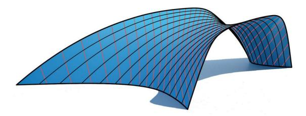
Figure 9. This saddle surface, a detail from the facade of the Cagliari Contemporary Arts Center, has been rationalized with 14 ruled surface strips. The strips have been simultaneously optimized towards a smooth overall surface under the constraint that the transition curves lie in user-specified vertical and coaxial planes.
