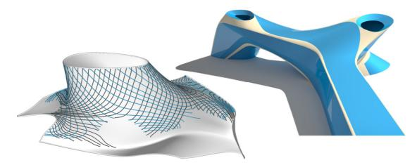
Figure 3. Curvature analysis yields a segmentation of the input shape into patches feasible for ruled surface approximation (right). The asymptotic curves follow the directions of vanishing normal curvature on a surface. In negatively curved (i.e., locally saddle shaped) regions there are two asymptotic directions in each surface point. If one family of asymptotic curves in a region is not curved too much, this indicates a good possibility for approximating that region by a ruled surface (left).
