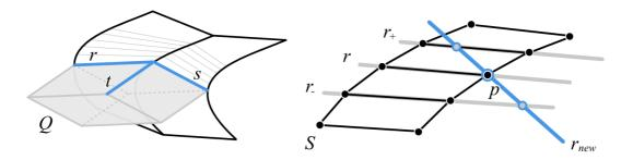
Figure 8. Tangent continuity of a ruled surface strip model implies vanishing volume of the parallelepiped Q spanned by the ruling directions r and s and the common boundary curve tangent t (left). The next strip's ruling in point p of a discrete curvature continuous strip model S is obtained as common intersection line  $r_{new}$  of r., r and  $r_+$  (right).
