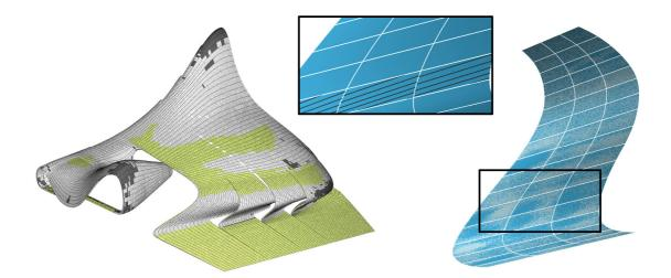
Figure 7. The panels of the Heydar Aliyev Cultural Centre facade by Zaha Hadid Architects are classified for planar (green), ruled (light grey) or general double curved (dark grey) rationalization (left). The ruled surface approximations of a subset of 51 panels are shown on the right, with some ruling directions visualized in a zoom-out (center).
