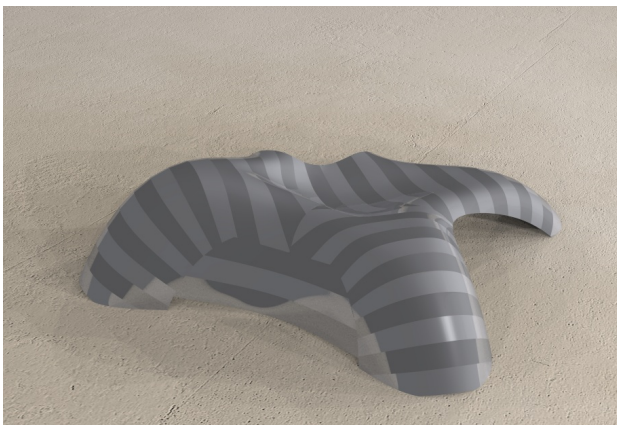
Figure 13: Watertight panels based on the segmentation and parallel transport methods. See also Figure 4. The intrinsic curvature of the rather broad panels is too high to make this design practicable: its purpose is to illustrate the parallel transport method.
