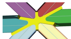
Figure 2: Node complexity. Manufacturing the connecting element (yellow) via plasma cutting requires much effort if the node has 'torsion', because of its truly spatial shape.
