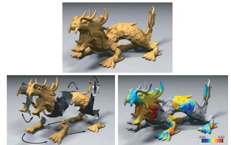
Approximate symmetry detection. (Top) Original sculpted dragon model, (left) detected partial and approximate symmetries, (right) color-coded deviations from perfect symmetry as a fraction of the bounding box diagonal.
