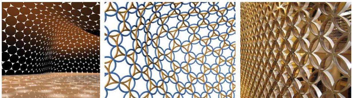
Left: Approximate circle packing of a freeform shape, derived from a CP mesh. Middle: CP meshes also serve as basis for the computation of freeform circle patterns; images: Alexander Schiffner. Right: A planar circle pattern in the Louis Vuitton store, Paris (image courtesy RFR).
