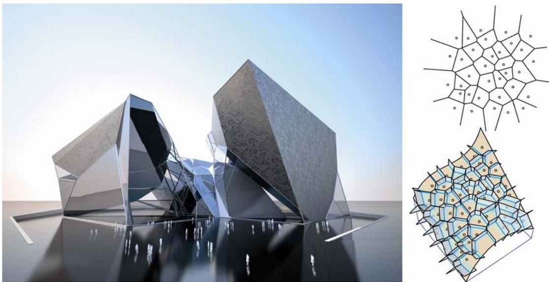
Voronoi diagrams associate nearest neighbor regions (Voronoi cells) to a set of input points. The concept works in the plane (upper right), for input points on a curved surface (lower right; only the part of the diagram close to the surface is shown) and in space (left; image courtesy B. Schneider). Voronoi diagrams and their numerous generalizations are a rich source for the design of spatial structures.
