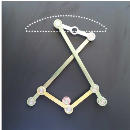
Approximate straight-line mechanism
