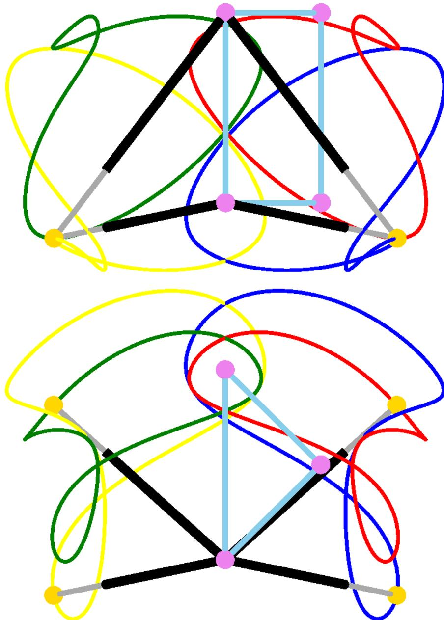
Figure 2: Side view and top view arranged as paired normal projections: The trajectories of the 1st resp. 2nd branch of the first anchor point (red resp. green) and fourth anchor point (blue resp. yellow).
