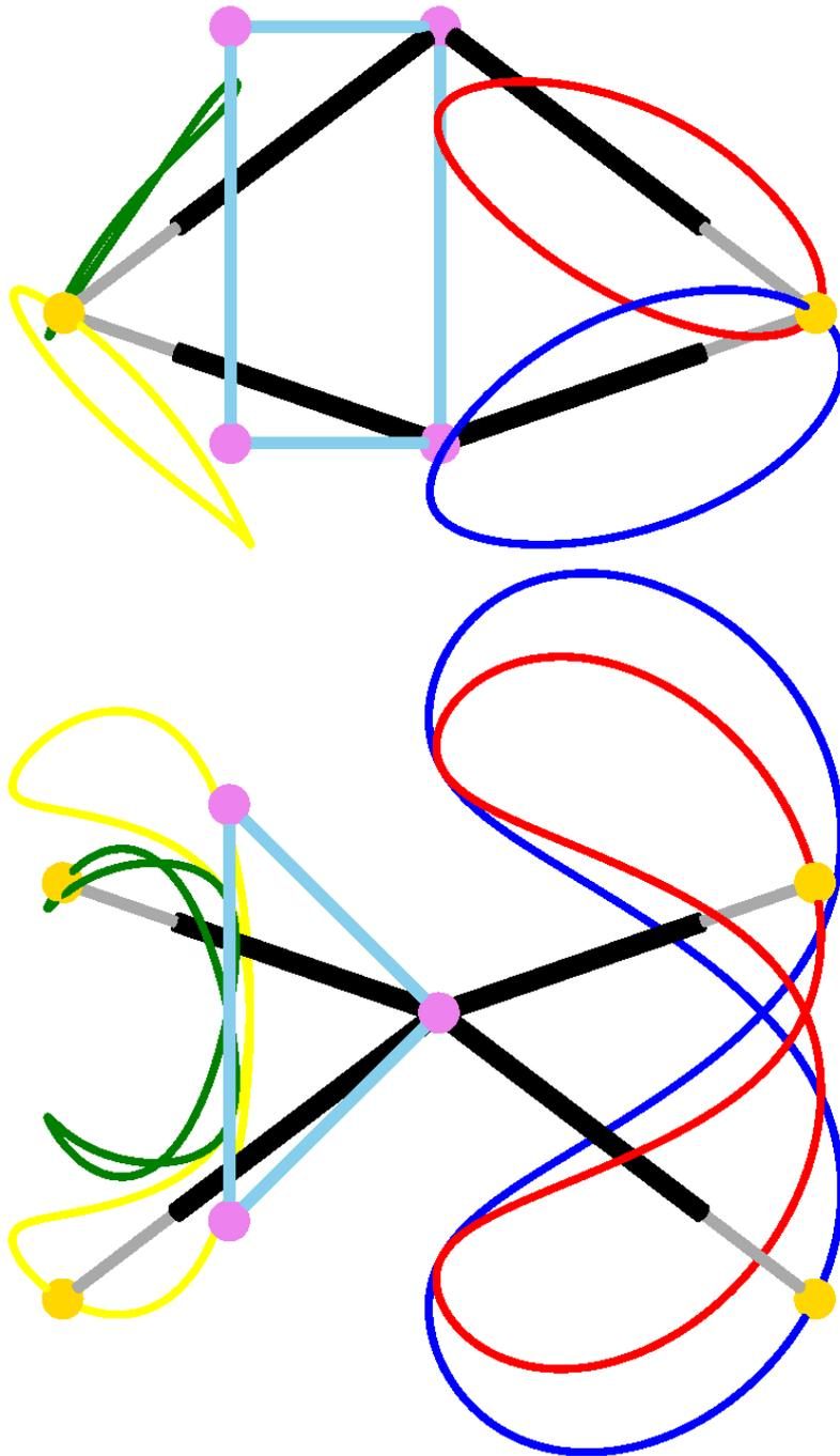
Figure 3: Side view and top view arranged as paired normal projections: The trajectories of the 1st and 2nd branch of the second anchor point (red and green) do not intersect each other. This also holds for the trajectories of the 1st and 2nd branch of the fifth anchor point (blue and yellow).
