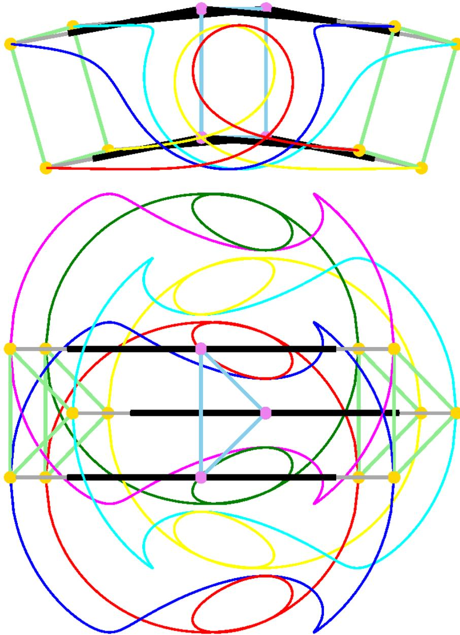
Figure 6: Side view and top view arranged as paired normal projections: The trajectories of the anchor points are colored in ascending order as follows: red, yellow, green, blue, cyan and magenta.
