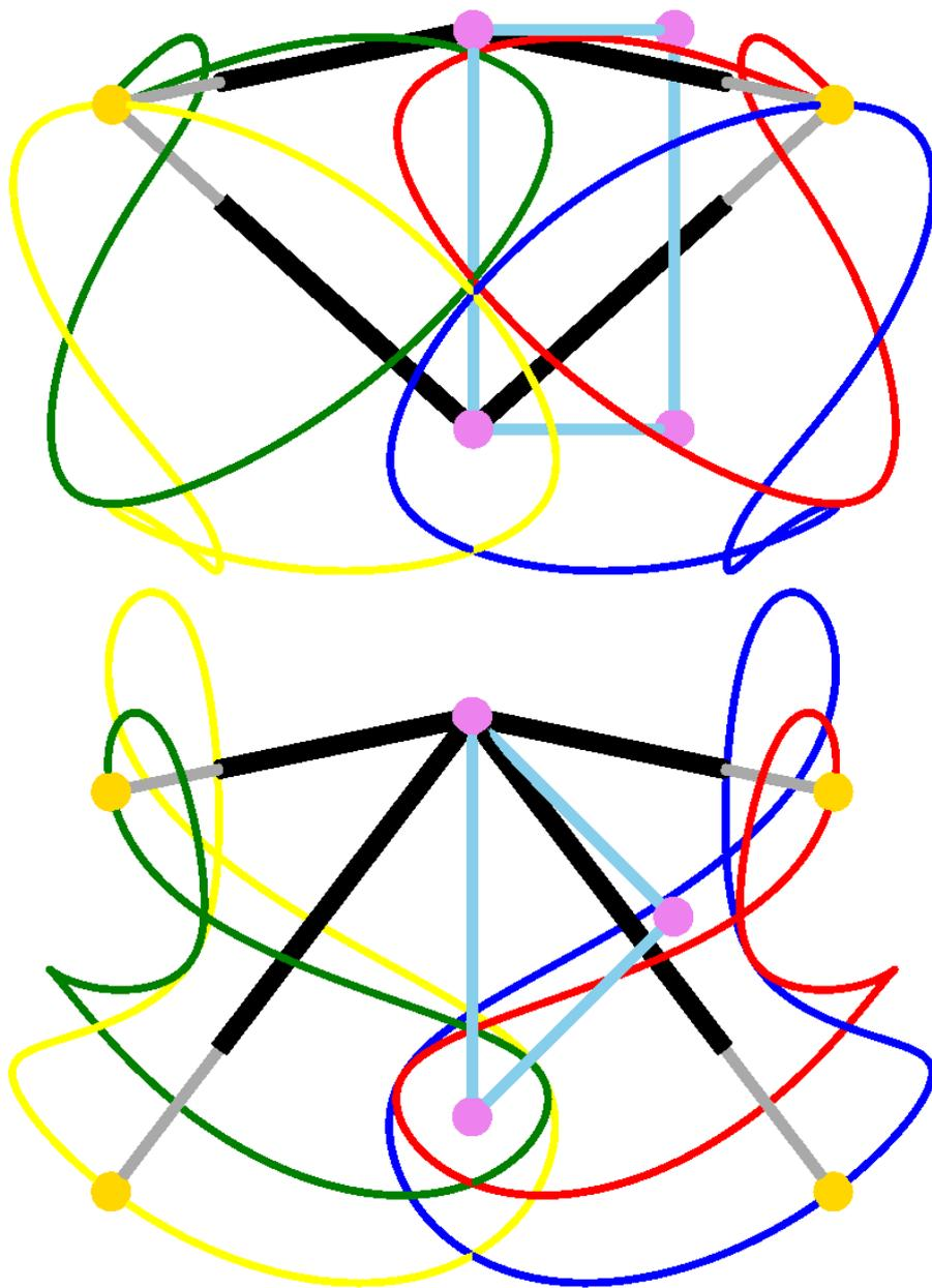
Figure 4: Side view and top view arranged as paired normal projections: The trajectories of the 1st resp. 2nd branch of the third anchor point (red resp. green) and sixth anchor point (blue resp. yellow).
