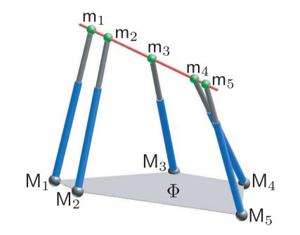
**Degenerated cases of (1a):** The 5 legs  $I_1, \ldots, I_5$  belong in any configuration with  $[m_1, \ldots, m_5] \parallel \Phi$  to a congruence of lines.
