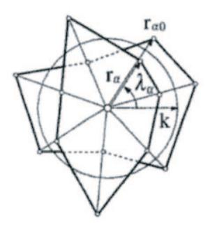
Wohlhart [2000] presented the *polygon platform*, i.e. the anchor points in  $\Phi$  and  $\varphi$ are related by an inversion.
