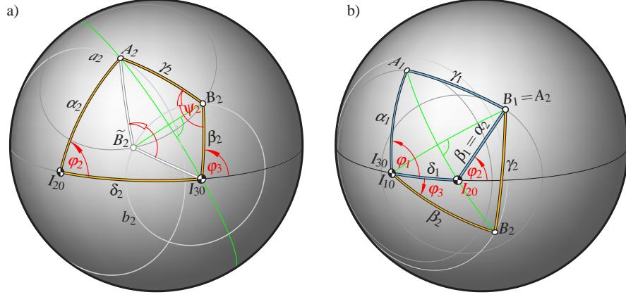
**Fig. 2** a) Opposite angles  $\phi_2$  and  $\psi_2$  at the second spherical four-bar  $I_{20}A_2B_2I_{30}$ .
