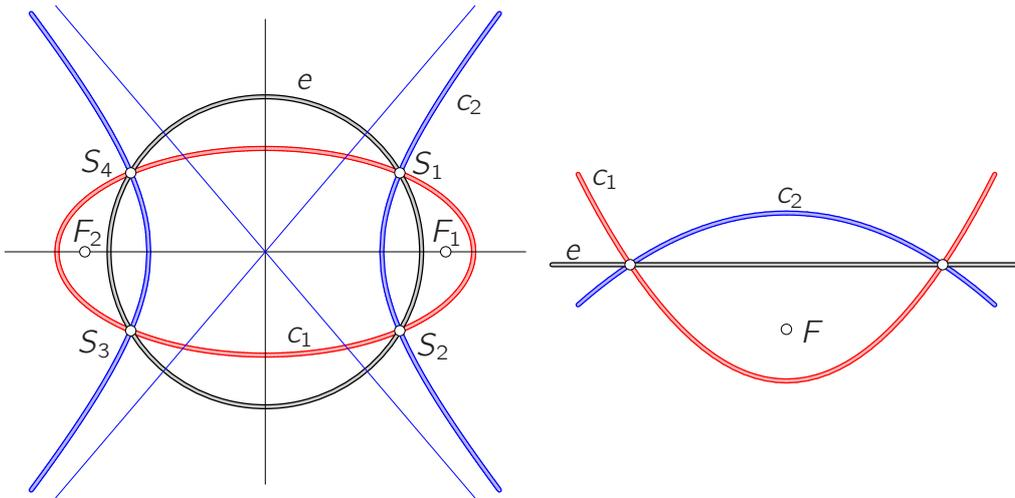
Figure 5: Equioptic curves of pairs of confocal conic sections.
