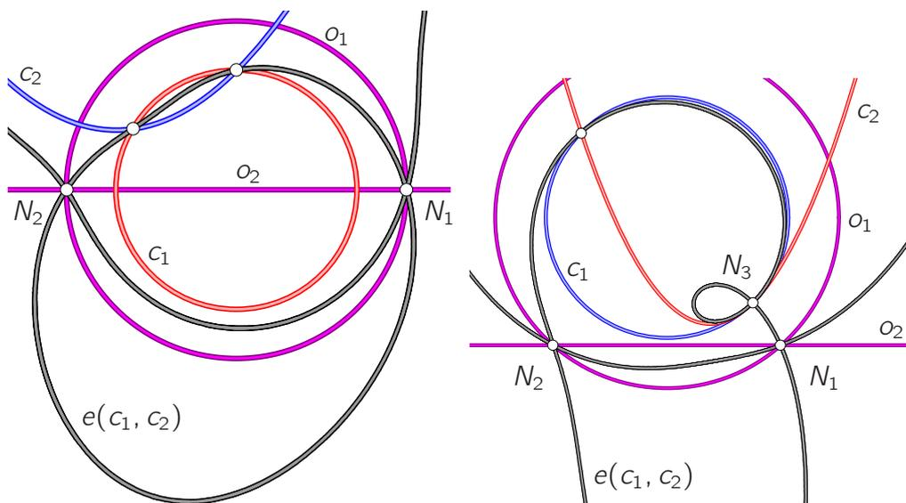
Figure 6: Singular points  $N_i$  on an equioptic curve  $e(c_1, c_2)$  of two conic sections. Left: Two conics in general position. Right: The equioptic of a parabola  $c_2$  with one of its osculating circles  $c_1$  has a further node at the point of osculation.
