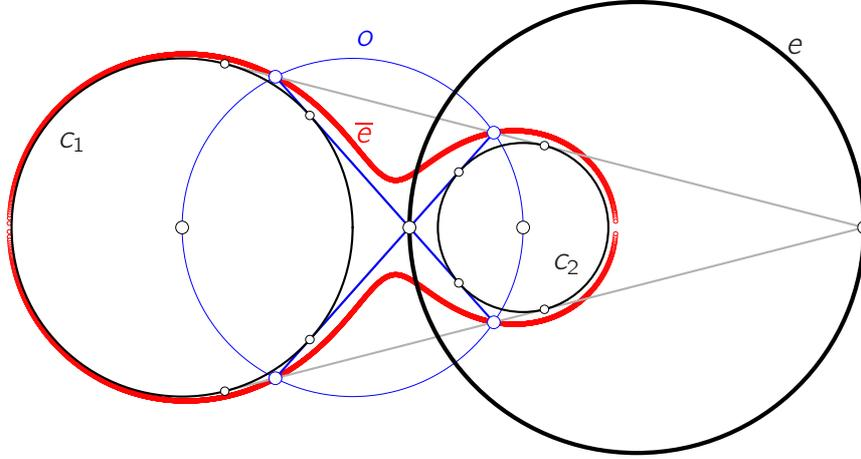
Figure 8: The quasi-equioptic curve  $\bar{e}$  of two circles is passing through the four intersection points of the common tangents of  $c_1$  and  $c_2$  but not through the centers of similitude.
