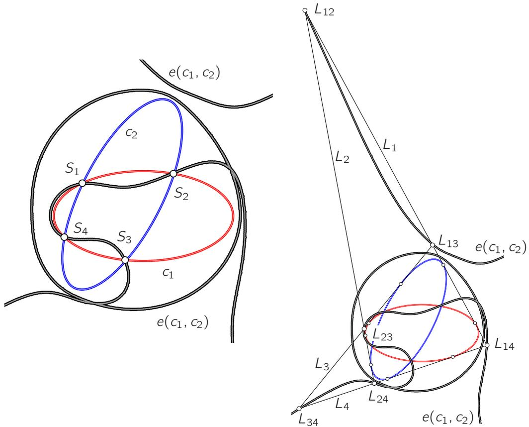
Figure 4: Left: The common points of  $c_1$  and  $c_2$  belong to  $e(c_1, c_2)$ . Right: The points  $L_{ij}$  of intersection of common tangents  $L_i$  and  $L_j$  of  $c_1$  and  $c_2$  are also contained in  $e(c_1, c_2)$ .
