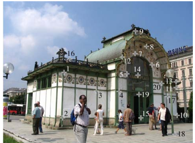
Fig. 3. Step 1) Specify pairs of corresponding points and determine their coordinates with respect to the camera frames
