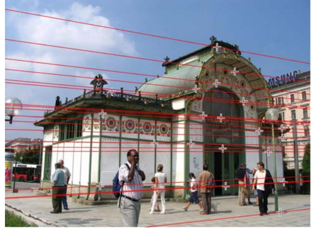
Fig. 4. Step 4) The essential matrix \mathbf{B} = \mathbf{S} \cdot \mathbf{R} determines the relative position of the two camera frames and hence the epipolar lines passing through the epipoles
