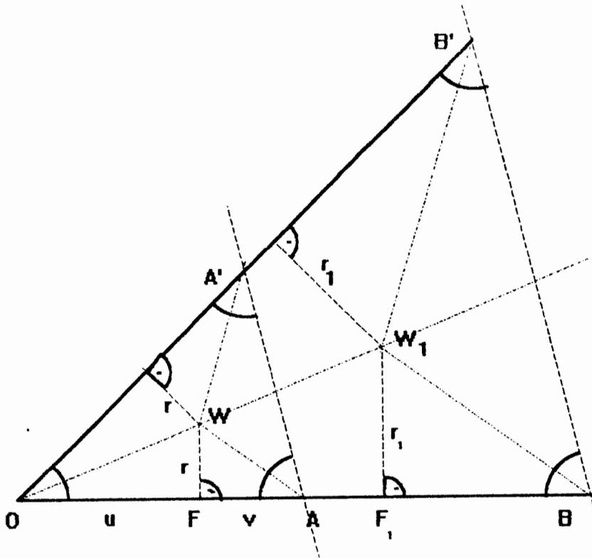
$$\left. \begin{array}{l} r:u = r_1:u_1 \Rightarrow r:r_1 = u:u_1 \\ r:v = r_1:v_1 \Rightarrow r:r_1 = v:v_1 \end{array} \right\} \Rightarrow \underline{u:u_1 = v:v_1} \Rightarrow (u+v):(u_1+v_1) = \underline{r:r_1} \Rightarrow a:b = r:r_1$$
