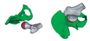
**Figure 6:** Partial Match: The goal is to fit a part (shown in purple) of the ball-joint to the hip-bone (shown in green). The starting arrangement (left) and the final alignment (right) are shown. The whole ball-joint is shown to help the reader judge the correctness of the match. Our algorithm is robust enough to handle varying sampling density and noise in the given PCDs.
