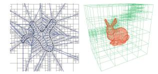
**Figure 2:** d2Tree can be used in 2D (left) and in 3D (right) to store quadratic approximants of the squared distance fields correct to some error threshold. The maximum number of levels and the error threshold, which are parameters used during the construction of this quad-tree like data-structure, determine the size of the cells. In the 2D case, we overlay the Voronoi diagram of the PCD on top of the d2Tree, to illustrate that small cells are created around the medial axis.
