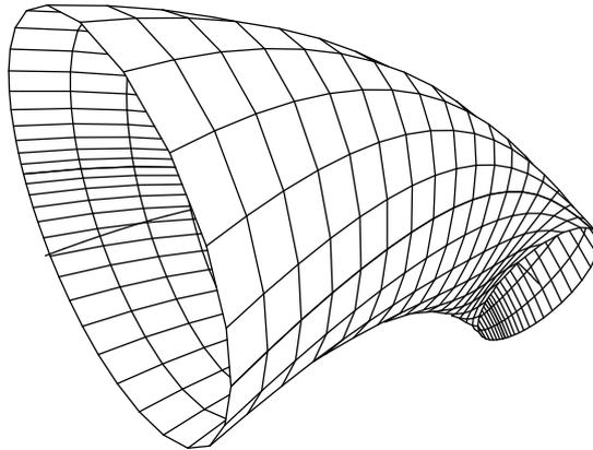
**Figure 5.** Canal surface defined by a cubic polynomial spine curve and a cubic polynomial radius.
