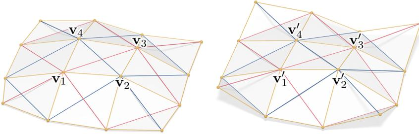
Figure 5: Isometric deformation of a surface represented as a quad mesh (yellow). In each pair of corresponding quads (in general not planar), corresponding diagonals (red, blue) have the same length and they form the same angle.
