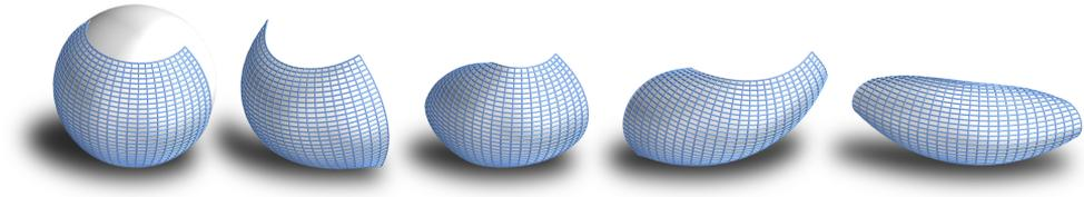
*Figure 1: Isometric deformations of a spherical patch. All these surfaces can be clad by bending panels formed on the same spherical mold. A sample building designed with these surfaces is shown in Fig. 2 (right).*
