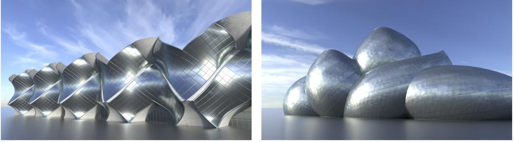
Figure 2: Architectural cladding with intrinsic repetition. On the left, a building composed by a repeated shape that is isometric to a Weingarten surface. For this kind of shapes, if dealing with flexible cladding materials,  $N$  panels can be formed with approximately  $\sqrt{N}$  molds and applied over the surface by isometric bending. On the right, a building made of surfaces isometric to the same sphere. In this case, all panels can be formed on a single mold and bent on the surface.
