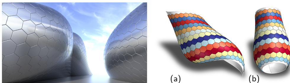
Figure 9: Hexagonal paneling with mold re-use. (a) A hexagonal panel layout designed on a shape isometric to a rotational surface. (b) For panel clustering and mold design, the panel layout shall be mapped back to the corresponding undeformed rotational surface. On the left, we illustrate shapes from Figures 4 and 1, clad with hexagonal flexible panels.
