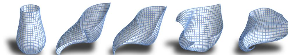
Figure 4: Isometric deformations of a rotational surface with (Wang et al., 2019). We can observe the high design freedom allowed by isometric deformations of a given shape.
