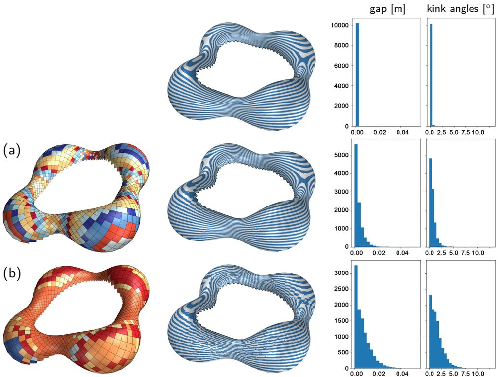
Figure 6: Comparison of paneling solutions on Weingarten surfaces obtained with (a) our method and (b) Eigensatz et al. (2010). The top row shows a solution with 960 unique cubic panels. From the left, the panels clusters and the resulting zebra striping of the panelized surface are shown. The histograms display the corresponding gaps and kink angles between adjacent panels, measured along the network of seam curves at 10216 regularly spaced locations. See Table 1 for further statistical data.
