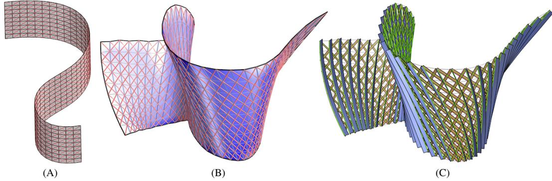
Figure 9: AGG-webs optimized from a developable surface. (A) A cylindrical AGG-web, which is isometric to a planar rectangular mesh with straight diagonals. (B) AGG-web obtained from the initial cylindrical web by interactive editing. The surface is colored by Gaussian curvature:  $K < 0$  (blue) and  $K = 0$  (white). (C) Designed AGG-web with developable strips.
