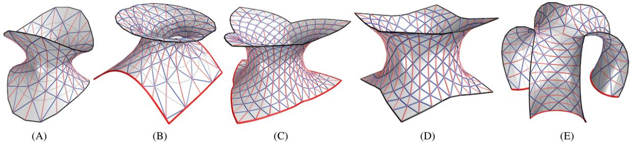
Figure 10: AAG-webs optimized from classical minimal surfaces. Part of their boundary curves (red) are constrained to be planar or linear. (A)-(B) Initial mesh from a *Scherk tower surface*. (B) Two bottom boundary curves are linear and another two planar. (C) Initialized from part of a *Schwarz H surface*. Bottom boundaries are coplanar. (D)-(E) Initial mesh from a *Schwarz P surface*. (E) Coplanar bottom boundary curves.
