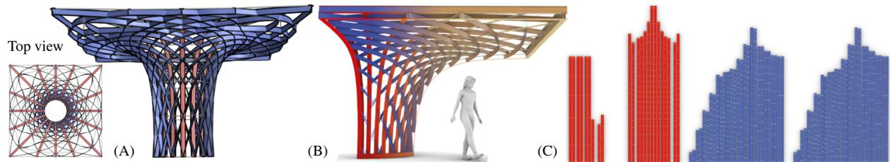
Figure 17: The timber roof structure was designed to be constructed exclusively from straight lamellas, including the edge and support beams. (A) Computed rotational AAG gridshell. Top and bottom mesh boundaries have square and circular shapes, respectively. (B) One quarter of the timber structure. (C) Developments with straight strips.
