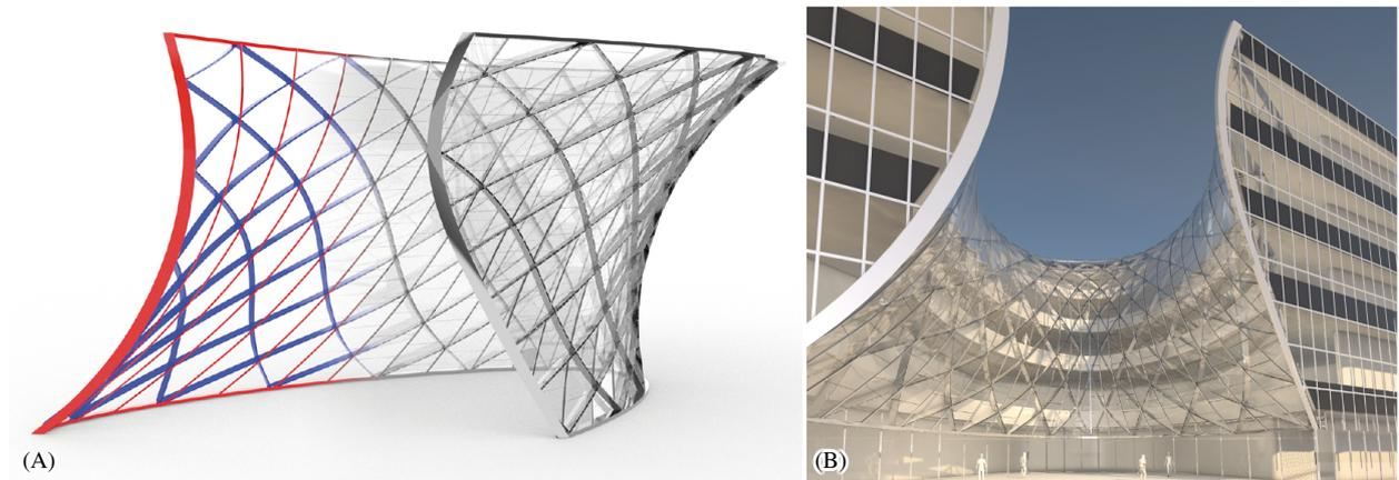
Figure 20: Architectural scenario of a doubly curved steel facade structure with developable glass panels. The design is inspired by the Emporia shopping Center Entrance in Malmö. (A) The strip geometry is used to generate a detailed architectural model of asymptotic double-lamellas, hinged joints and developable facade panels. (B) The facade is integrated as semi courtyard in a rectangular building block.
