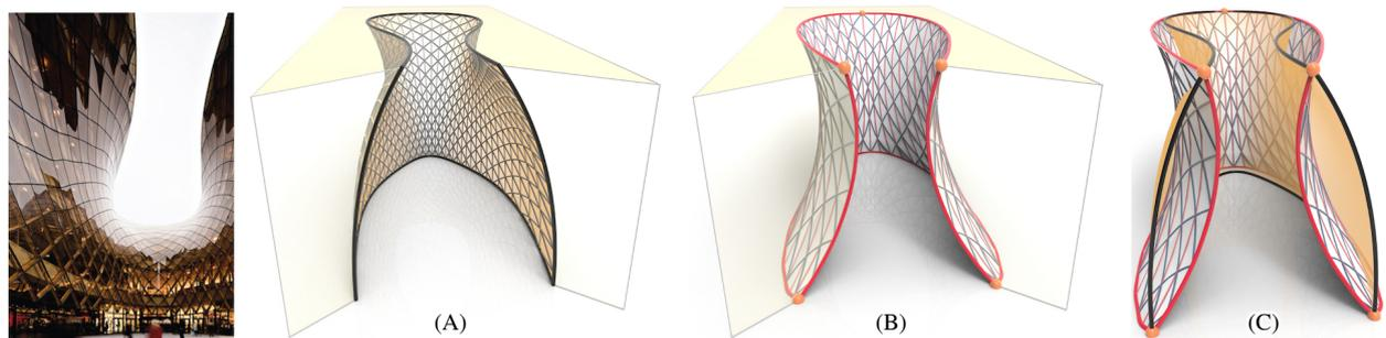
Figure 19: Optimization workflow for the Emporia Shopping Center facade: (A) Original mesh with four planar boundaries. (B) Optimized AAG-web with fixed points and boundaries gliding on the same original planes. The strips are shown in Fig. 20(A). (C) Comparison of meshes (A) and (B).
