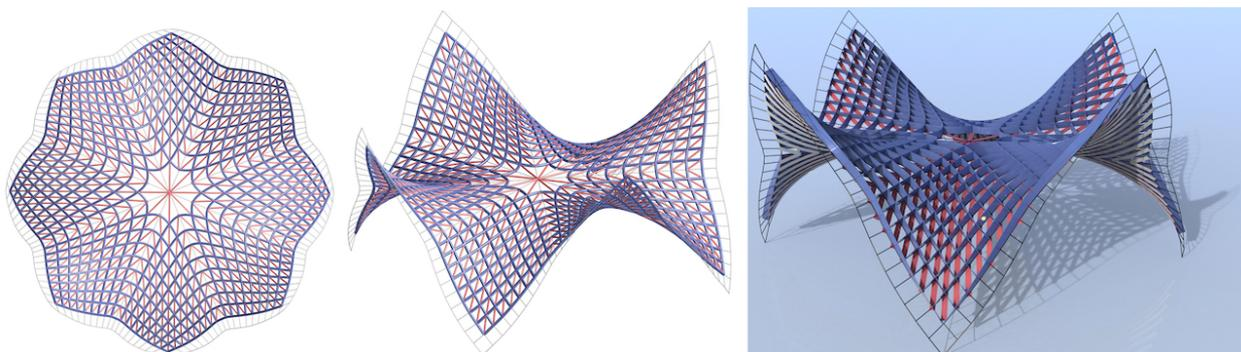
Figure 14: An AAG gridshell with a central combinatorial singularity. Diagonal geodesics break at eight polylines through the singularity.
