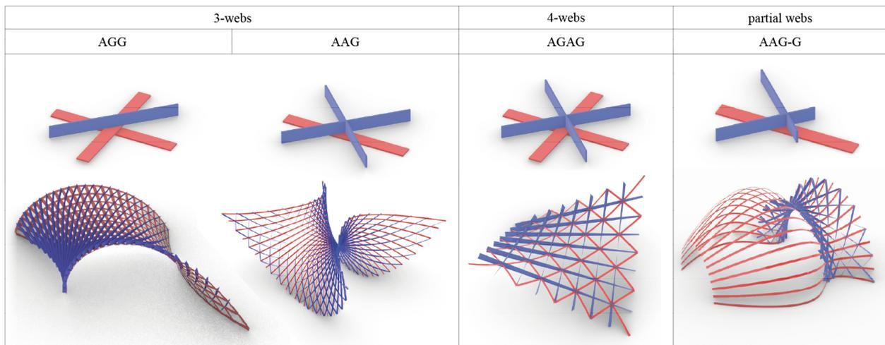
Figure 4: Overview of the possible 3- and 4-webs combining asymptotic (A,blue) and geodesic (G,red) lamellas. Partial webs may extend the geodesic network onto surface regions of positive curvature.
