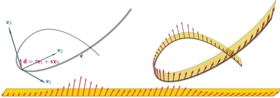
Figure 5: Left: The Darboux vector  $\mathbf{d}$  in the rectifying plane of the Frenet frame attached to a space curve  $\mathbf{c}$ . Right: The Darboux vectors at all curve points define the rulings of the rectifying developable surface  $D$  through  $\mathbf{c}$ . Bottom: In the planar development of  $D$ , the curve  $\mathbf{c}$  lies in a straight line.
