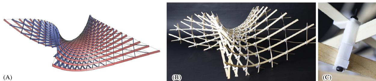
Figure 12: The computed mesh (A) was used to create a physical verification model (B). For this purpose, straight slats were connected laterally with hinged 3D joints.
