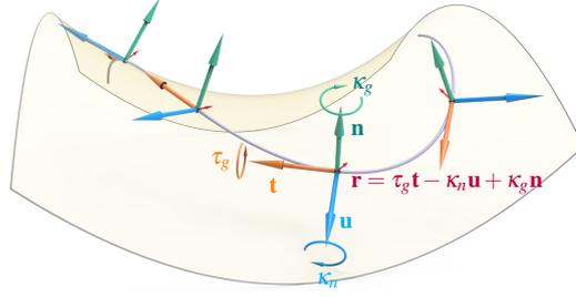
Figure 6: The Darboux frame depicting the three “curvatures”  $\tau_g$ ,  $\kappa_n$ ,  $\kappa_g$  of a curve on a surface.
