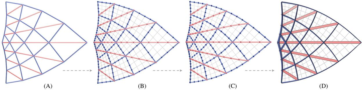
Figure 7: Overview of the computational approach. (A) coarse web (here, an AAG-web; A=blue, G=red). (B) refined web after applying subdivision twice. (C) relevant polylines on the refined mesh are optimized so that they possess the required properties (asymptotic or geodesic). (D) AAG network from three families of developable strips.
