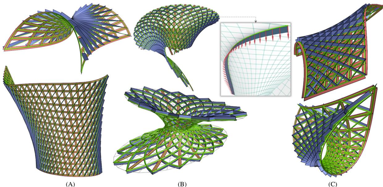
Figure 13: Digital models of various types of asymptotic geodesic hybrid gridshells. Column (A) AGG-webs, column (B) AAG-webs, column (C) AGAG-webs with low numerical errors (see Table 2). A zoom onto one strip, orthogonal to the reference surface, together with the ruling vectors is also shown.
