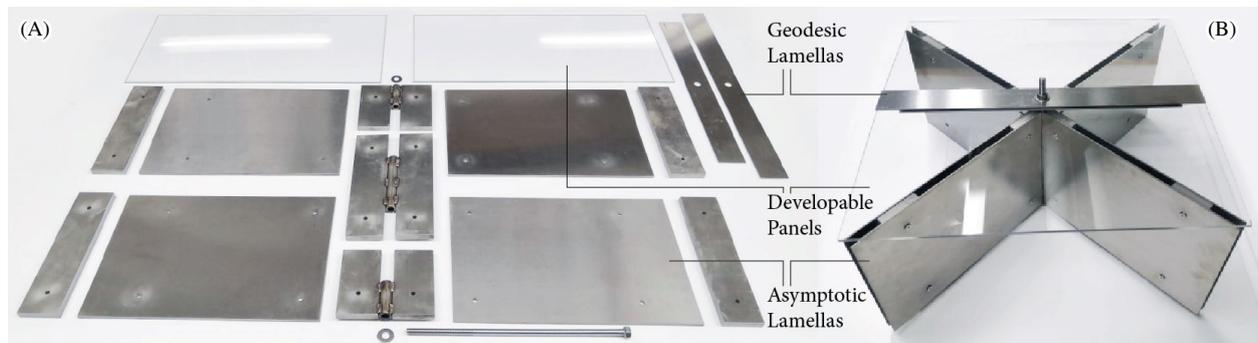
Figure 21: Prototypical steel joint for the doubly curved facade structures (B). All elements can be unrolled flat and straight (A). The asymptotic lamellas are segmented and connected at each intersection through a hinged scissor joint that adjust to the individual intersection angle. The geodesic lamellas acts as the outer mullion system that clamps the developable glass panels.
