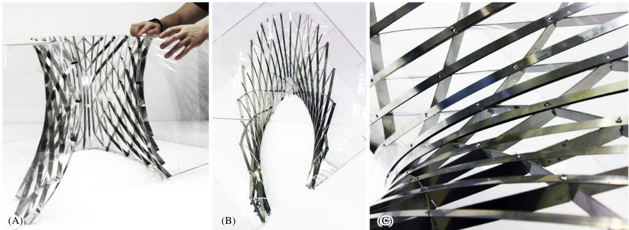
Figure 22: Steel model of the optimized AAG facade structures at scale 1:20, shown in elevation (A), plan (B) and close-up view (C). The two asymptotic families are constructed with slots in the same level. The geodesic lamellas function as triangulation and substructure for the transparent facade panels.
