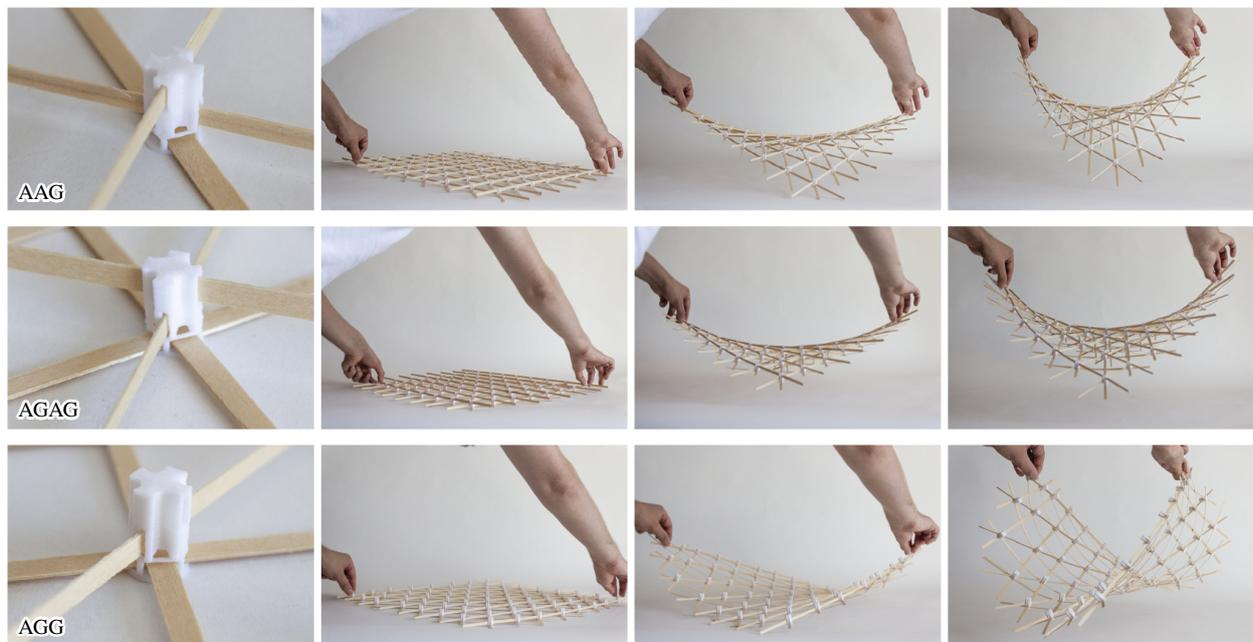
Figure 15: Physical deformation experiment for equilateral AG-webs. AAG- and AGAG-webs naturally deform into a negatively curved shape. AGG-webs naturally seek a nearly developable shape. A similar deformation of an AAG-web was simulated digitally (see Fig. 16)
