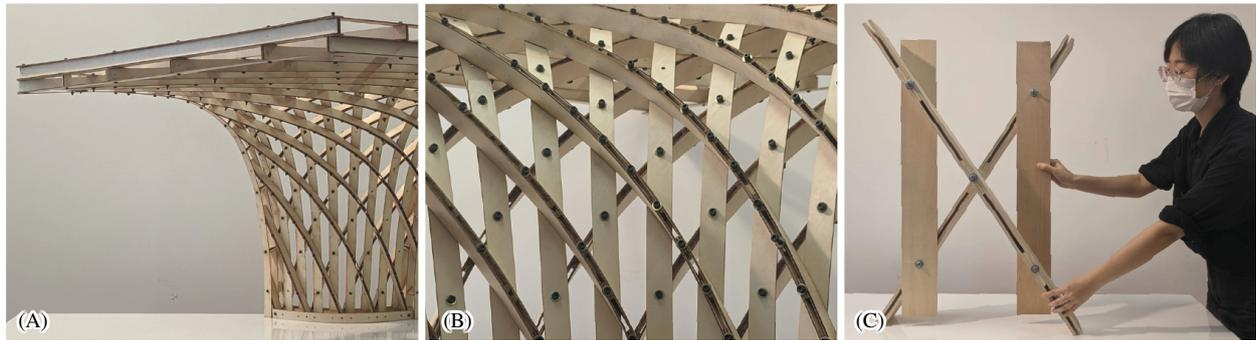
Figure 18: A timber prototype was constructed at 1:5 scale (80 x80 cm). The combination of double asymptotics and interwoven geodesics create a strong web, halves the buckling length and braces the structure. A 1:1 joint was built to test the laminated joints, and bolt connections.
