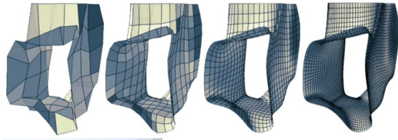
Figure 11: Quad meshing the Opus project by Zaha Hadid architects using subdivision and PQ optimization. This works better than our analytic method because of large almost-flat areas where conjugacy is numerically unstable and misleading (image from the survey paper [PSW08]).
