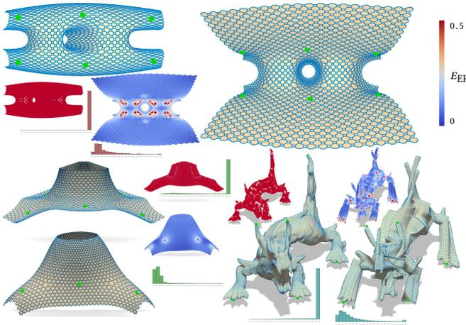
Fig. 15. Meshes optimized for Euclidean regularity. Top and bottom left: the optimized geometry for these semi-regular patterns. Note that they appear as if made from conic patches, as the original patterns are planar. Bottom right: the optimized dragon exhibits a shape that is made from patches that are as developable as possible, having the appearance of a “paper toy”.
