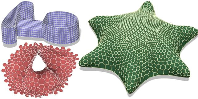
Fig. 5. Meshes optimized for Euclidean regularity. The quad mesh assumes perfect developability, the heptagonal mesh assumes a hyperbolic pattern, as the prescribed angle defect is negative, and the hexagonal mesh has the appearance of a dual geodesic dome.
