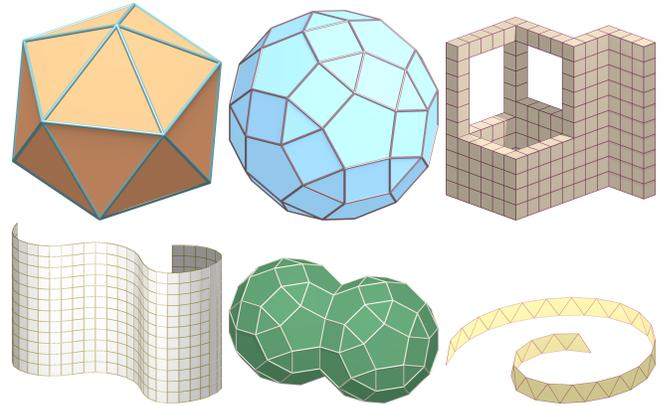
Fig. 4. Perfect Euclidean-regular meshes. Top row: Icosahedron (left), Archimedean solid (rhombicosidodecahedron; center), PolyCube mesh (right). Bottom row: developable quad mesh (left), two Archimedean solids glued together (center), developable triangle strip (right).
