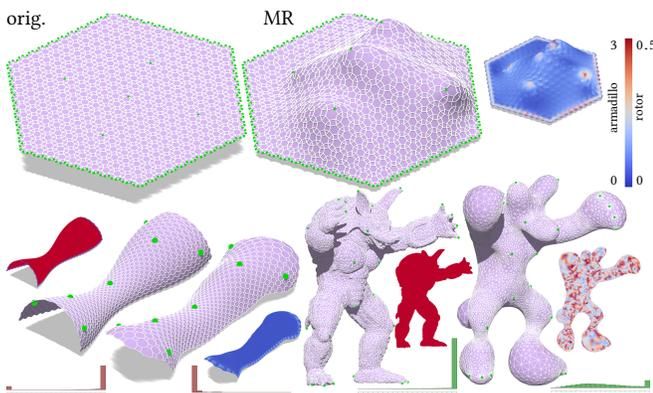
Fig. 14. Meshes optimized for Möbius regularity with direct optimization. Top: designing a Möbius regular shape from a patch of the (6, 4, 3, 4) pattern by prescribing position constraints (green dots). Bottom: optimizing existing designs. Left: a (12, 6, 4, 6) pattern. Right: a triangle mesh, giving the appearance of a “blob toy”. The colors refer to the  $E_{MR}$  energy per vertex.
