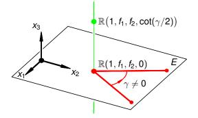
The rotation about the fixed point  $\mathbb{R}(1, f_1, f_2, 0)$  through the angle  $\gamma \neq 0$  is mapped to the point  $\mathbb{R}(1, f_1, f_2, \cot(\gamma/2))$ .
