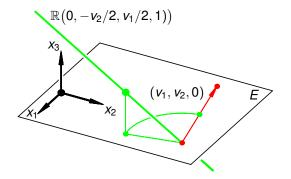
The translation along the vector  $(v_1, v_2, 0)$  is mapped to the point  $\mathbb{R}(0, -v_2/2, v_1/2, 1)$ , which belongs to the plane at infinity.
