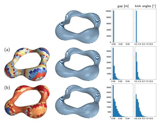
Figure 6: Comparison of paneling solutions on Weingarten surfaces obtained with (a) our method and (b) Eigensatz et al. (2010). The top row shows a solution with 960 unique cubic panels. From the left, the panels clusters and the resulting zebra striping of the panelized surface are shown. The histograms display the corresponding gaps and kink angles between adjacent panels, measured along the network of seam curves at 10216 regularly spaced locations. See Table 1 for further statistical data.
