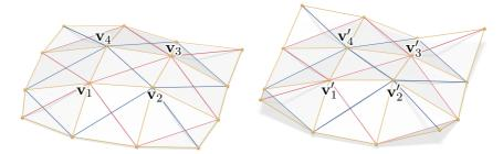
Figure 5: Isometric deformation of a surface represented as a quad mesh (yellow). In each pair of corresponding quads (in general not planar), corresponding diagonals (red, blue) have the same length and they form the same angle.
