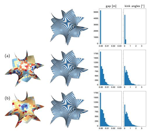
Figure 7: Comparison of paneling solutions on Weingarten surfaces obtained with (a) our method and (b) Eigensatz et al. (2010). The top row shows a solution with 480 unique cubic panels. From the left, the panels clusters and the resulting zebra striping of the panelized surface are shown. The histograms display the corresponding gaps and kink angles between adjacent panels, measured along the network of seam curves at 5336 regularly spaced locations. See Table 1 for further statistical data.
