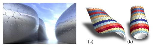
Figure 9: Hexagonal paneling with mold re-use. (a) A hexagonal panel layout designed on a shape isometric to a rotational surface. (b) For panel clustering and mold design, the panel layout shall be mapped back to the corresponding undeformed rotational surface. On the left, we illustrate shapes from Figures 4 and 1, cladded with hexagonal flexible panels.
