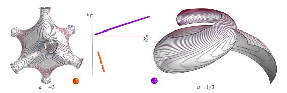
Figure 17: Alignment of isolines of principal curvatures  $\kappa_1$  and  $\kappa_2$ , respectively (blue,red) on two discrete CRPC surfaces. The estimated principal curvature values yield points on the correct straight lines in the  $(k_2, k_1)$ -plane.
