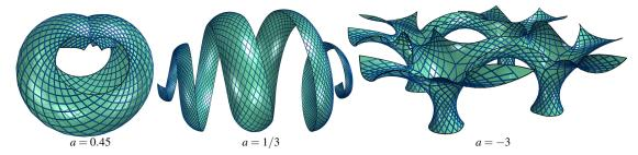
Figure 20: Discrete CRPC surfaces, optimized after joining copies of smaller CRPC meshes. *Left:* a = 0.45, initial piece from Fig. 1. *Center:* a = 1/3, initial shape from Fig. 17, right. *Right:* Input mesh obtained from Fig. 18 with  $2\gamma = 60^{\circ}$  by cutting it, joining four copies and editing the whole shape.
