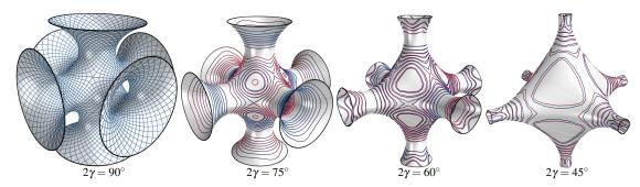
Figure 18: Discrete negatively curved CRPC surfaces with selected curvature isolines, obtained from a discrete minimal surface (A-net with  $2\gamma = 90^{\circ}$ ) by keeping the mesh combinatorics and optimizing for other angles in the A-net.
