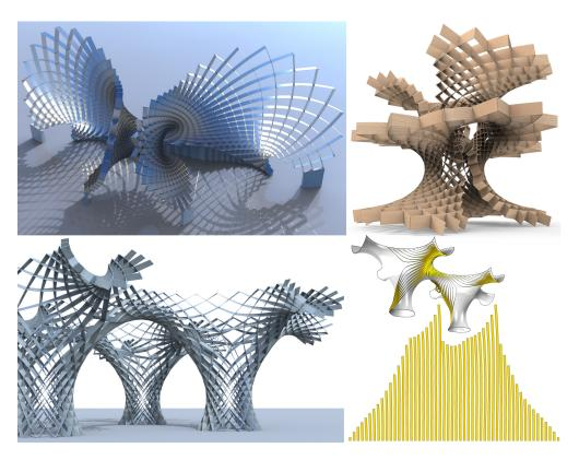
Figure 22: Asymptotic gridshells, formed by developable surface strips with a straight development, that are attached orthogonally to negatively curved CRPC surfaces along selected asymptotic curves. *Top*: Gridshells from minimal surfaces, a = -1. *Bottom*: Gridshell with node angle  $\pi/3$ , a = -3. Even in this coarse discrete model for the strips, their development is nearly straight.
