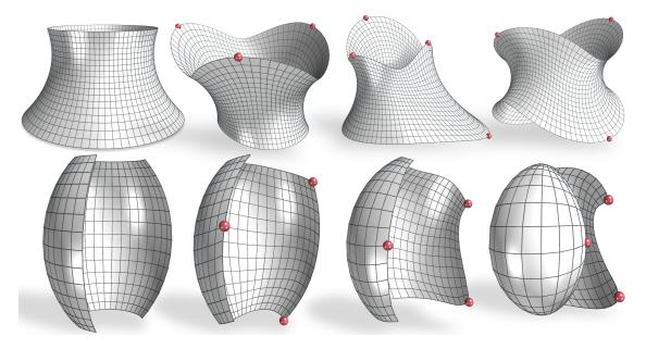
Figure 19: Modeling CRPC surfaces through mesh editing. We start from meshes representing rotational CRPC surfaces (top left:  $\gamma = 38.5^{\circ}$ , bottom left: a = 2) and drag some vertices to new locations. The curvature ratio a is fixed and the shown meshes are the control meshes for the diagonal mesh approach.
