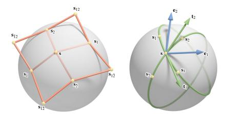
Figure 8: Left: In an S-net, any central vertex s and its four neighbors  $s_1, s_2, s_{\bar{1}}, s_{\bar{2}}$  lie on a common sphere. Right: Discrete osculating circles of the two discrete parameter lines through a vertex. The bisecting vectors  $e_1, e_2$  of their tangent vectors  $t_1, t_2$  are the discrete principal directions (images from [2]).
