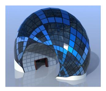
Figure 1: Architectural design study exhibiting a structure from planar panels based on a discrete CRPC surface with a=0.45. The constant node angle  $(\neq \pi/2)$  and the principal symmetric arrangement lead to a more interesting visual appearance than a mesh aligned with principal curvature directions would have.
