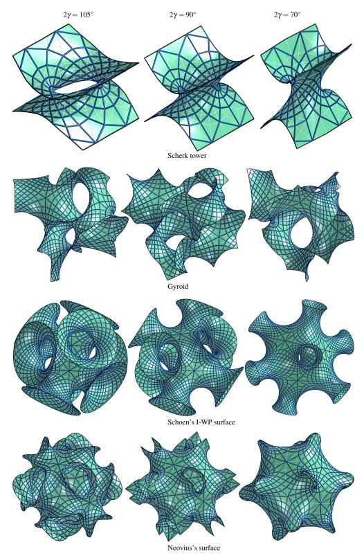
Figure 21: Discrete CRPC surfaces obtained from selected classical minimal surfaces (center) by changing the angle  $\gamma$  in the A-net.
