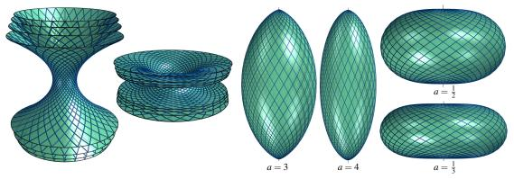
Figure 5: Rotational CRPC surfaces. Left: a = -2, -3, -4, -5 and  $a = -\frac{1}{5}, -\frac{1}{4}, -\frac{1}{3}, -\frac{1}{2}$  from outside to inside. Right:  $a = 3, 4, \frac{1}{2}, \frac{1}{3}$ .
