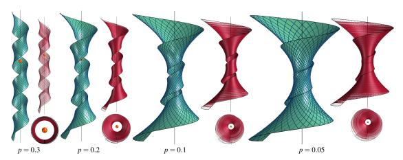
Figure 14: Discrete helical CRPC surfaces with a=-3 and decreased pitch p=0.3,0.2,0.1,0.05. The boundary curves of the surfaces arise from the used control net and are diagonal to the net of characteristic curves.
