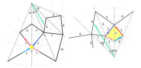
Figure 11: Radially symmetric nets as reciprocal force diagrams.
