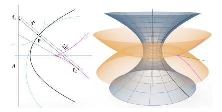
Figure 6: A well-known construction of the curvature centers  $\mathbf{f}_2$  of a parabola (left) from the intersection points  $\mathbf{f}_1$  of its normals with the directrix A shows that the surface obtained by rotating a parabola about its directrix A has a constant negative ratio of principal curvatures  $\kappa_1/\kappa_2 = -2$ . We also show the evolute of the parabola, which generates the nontrivial part of the focal surface of the CRPC surface.
