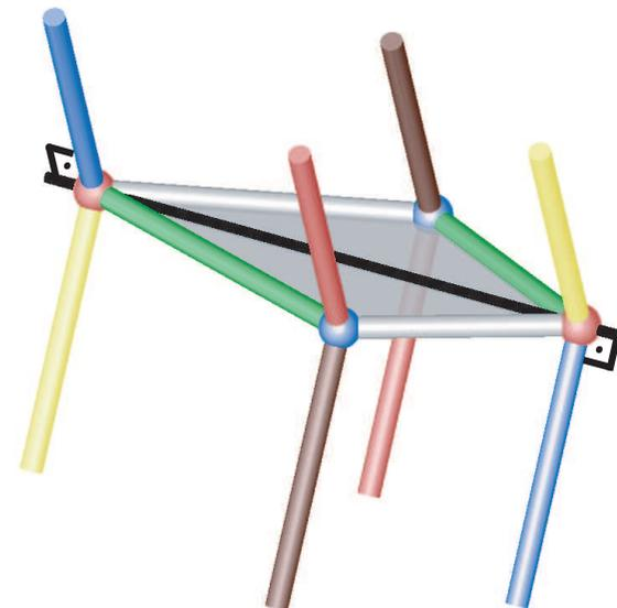
For the special case of coinciding faces during the flex, we get again the *butterfly motion* and the *spherical four-bar motion*.
