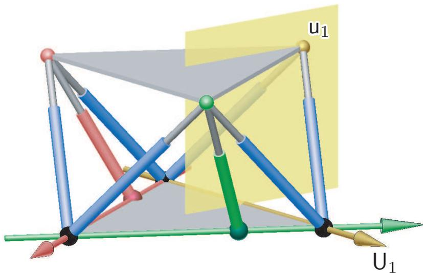
The **Mannheim constraint** that a plane of  $\Sigma$  orthogonal to  $u_j$  slides through the point  $U_j \in \Sigma_0$  is a homogeneous quadratic equation  $\Pi_j$  in the Study parameters ( $j = 4, 5, 6$ ).
