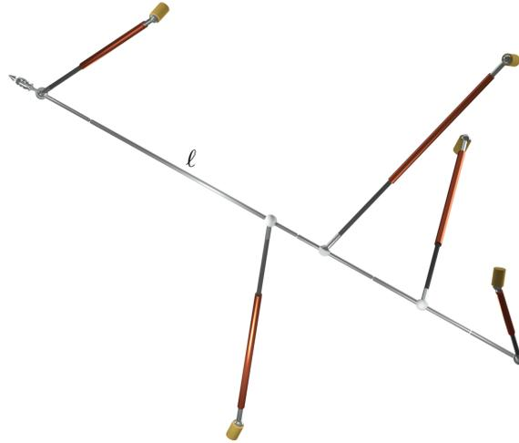
It turns out that this kind of manipulator is an interesting alternative to serial robots handling axis-symmetric tools. Some fundamental industrial tasks such as 5-axis milling, laser engraving and water jet cutting can be counted as its applications in industry.
