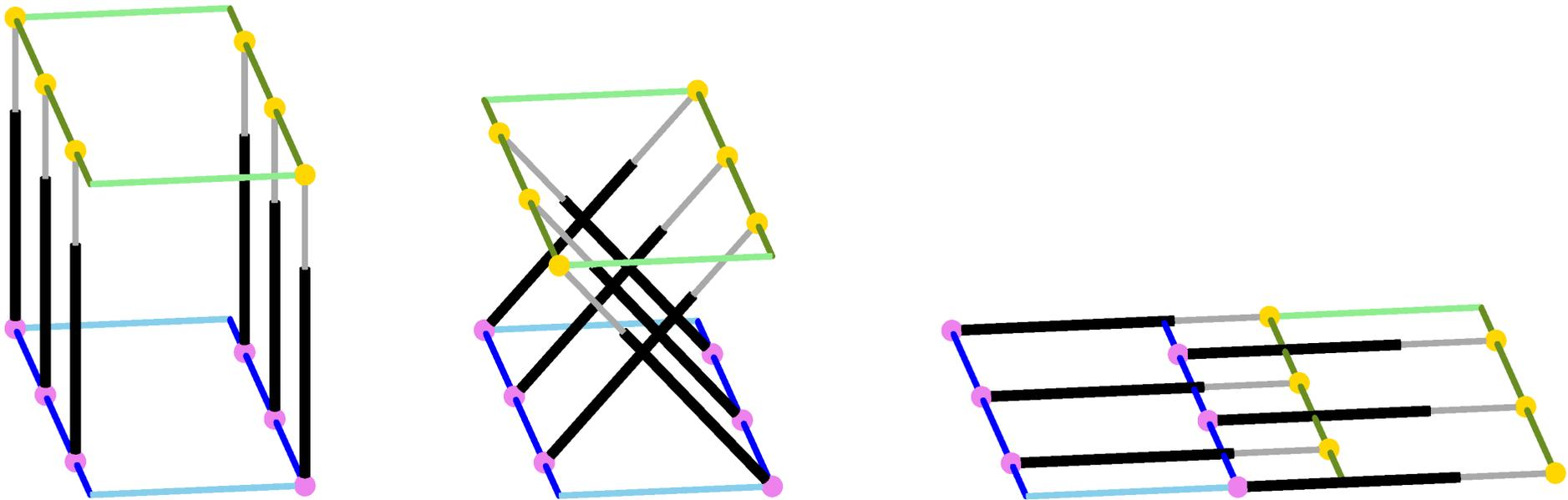
We study a congruent SGP, where the anchor points are located on the  $x$ -axis and a parallel line through  $(0, d, 0)$ . Therefore the manipulator is architecturally singular. If all legs have equal lengths, this manipulator has two 2-dimensional self-motions.
