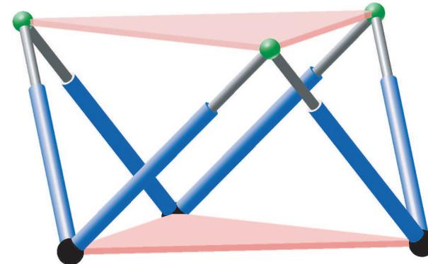
A SGP is a parallel manipulator where the platform is connected via three Spherical-Prismatic-Spherical (SPS) legs with the base.
