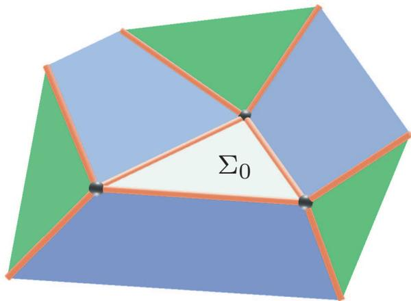
A Kokotsakis mesh is a polyhedral structure consisting of a  $n$ -sided central polygon  $\Sigma_0$  surrounded by a belt of polygons.
