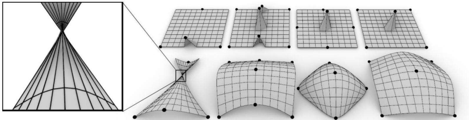
A crucial assumption is the smoothness of the output mesh. The formulation of our fairness term does not support the generation of anti-V-hedra or hybrid versions.
