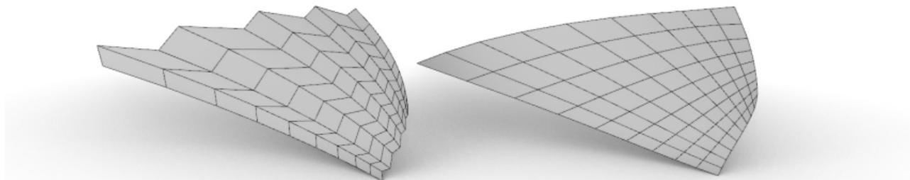
Given an input quad mesh and we optimize for face planarity, fairness, and (anti-)Voss property; while the corners are fixed. The implemented iterative algorithm is based on
