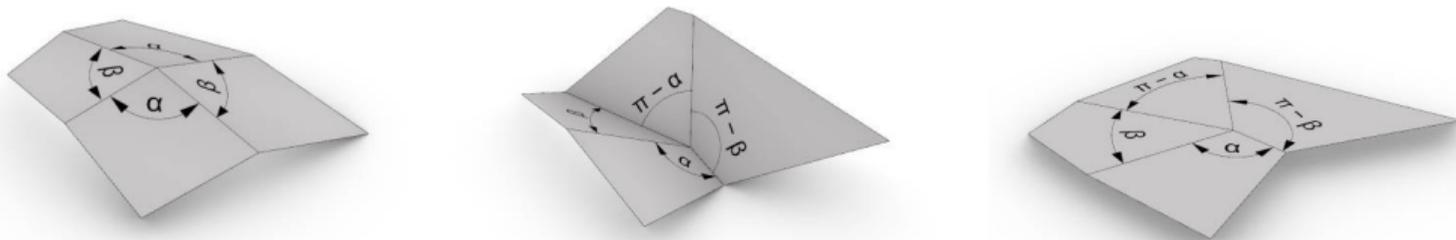
The geodesic condition translates into the equality of opposite angles at every vertex.
