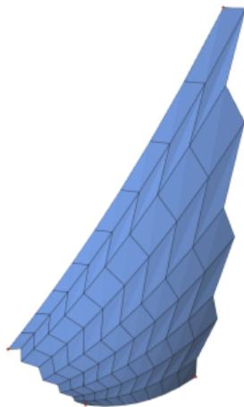
Discretization plus random noise. Input of the Approximation Algorithm.
