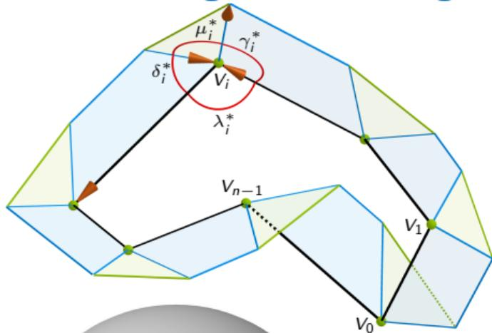
The spherical image of faces around two adjacent vertices  $V_i$  and  $V_{i+1}$  corresponds to two coupled spherical 4-bar mechanisms.
