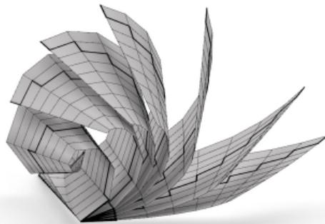
**Open problem:** How to assign the two possible normals to the faces in such a way that the resulting surface has no self-intersections and is close to some desired geometry?
