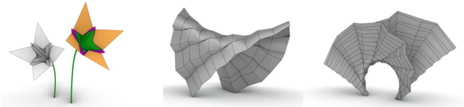
There is no need for this convexity restriction as it limits the design space artificially. For the same reason we allow flipped quads, which additionally enables us to discretize some surface singularities\* without introducing vertices with a valence different than four.
