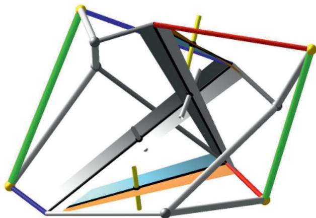
**Remark:** The corresponding 6R loops in the flexible arrangement of two Bennett tubes of families (A) and (B) are line-symmetric.
