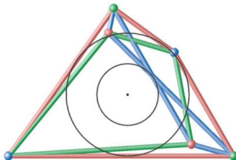
**Bricard octahedra** can also be seen as flexible bipyramids, where each quadrilateral pyramid corresponds to a spherical 4R-loop.
