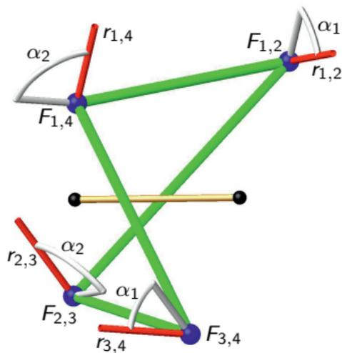
As pointed out by Hon-Cheung\* **Bennett loops are line-symmetric** (if neglecting the orientation of the rotation axes). Therefore the relative motion of opposite links is line-symmetric, which was intensively studied by Krames†.
