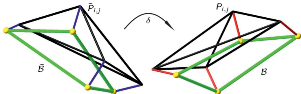
$\mathcal{B}$  and  $\bar{\mathcal{B}}$  can be flexible coupled over the two tetrahedra  $P_{1,4}, \dots, P_{3,4}$  and  $\bar{P}_{1,4}, \dots, \bar{P}_{3,4}$  if for each  $\tau$  there exists a  $\bar{\tau}$  such that the two tetrahedra are related by an isometry  $\delta$ .
