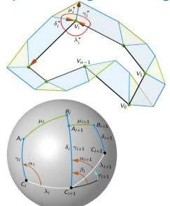
The spherical image of faces around two adjacent vertices  $V_i$  and  $V_{i+1}$  corresponds to two coupled spherical 4-bar mechanisms.
