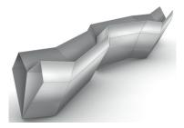
Therefore the zip row has the property that two planar polylines remain planar during its isometric deformation.
