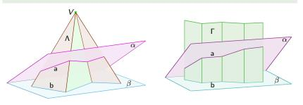
**1.** planes parallel to  $\alpha$  (resp.  $\beta$ ) also carry curves of  $\Lambda$  and  $\Gamma$ , respectively, which remain planar during  $\iota$ .
