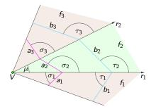
We consider  $f_2$  as fixed and locate it in the *xy*-plane of the reference frame such that *V* equals the origin and  $r_1$  coincides with the *x*-axis.
