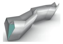
Consist of two T-tubes which can be glued together along the zip row such that the resulting structure is still rigid-foldable.
