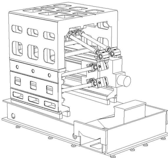
Figure 2: A three-axes version of a parallel manipulator for translatory movement
