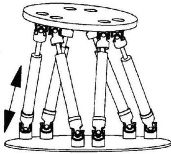
Figure 1: Example of a parallel manipulator
