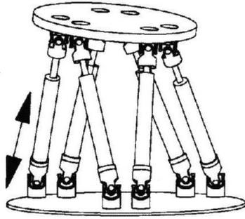
Figure 1: Example of a parallel manipulator
