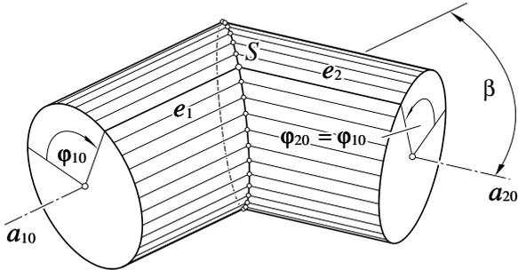
Figure 6: The condition for uniform transmission
