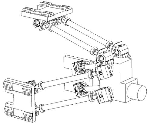
Figure 3: The skeleton of this manipulator
