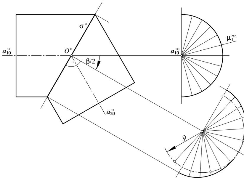
Figure 7: Auxiliary view showing the bisector plane  $\sigma$  in true size
