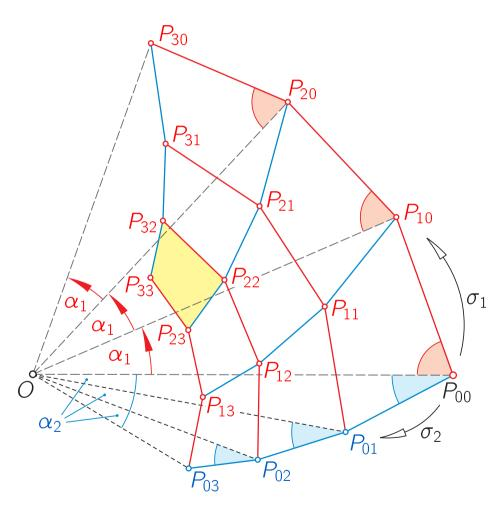
Given: two stretch-rotations  $\sigma_1$ ,  $\sigma_2$  with common center O, with respective signed angles  $\alpha_1$ ,  $\alpha_2$  of rotations and dilation factors  $\delta_1$ ,  $\delta_2 \neq 1$ .
