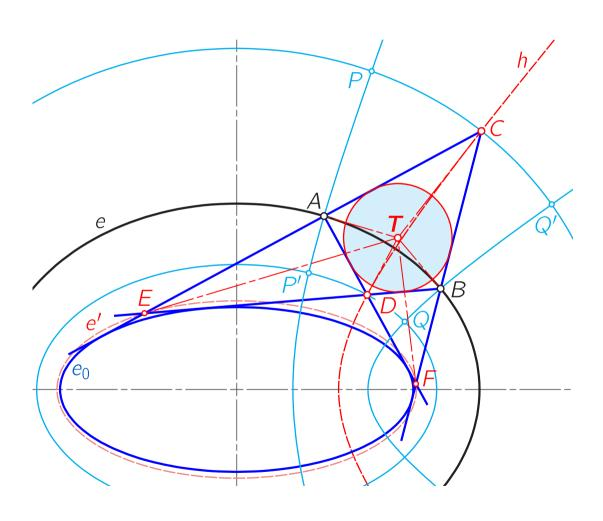
The tangents at A, B to e, at E, F to e' and at C, D to h pass through point T.
