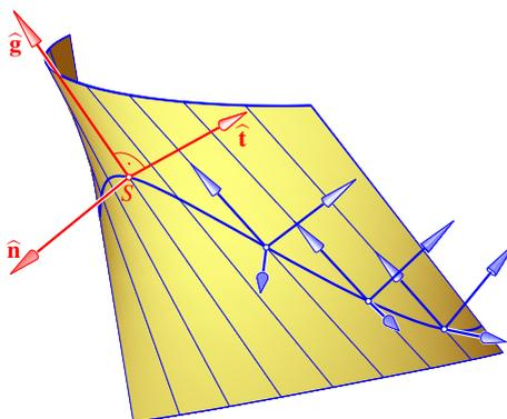
Figure 2: Frenet frame  $(\widehat{\mathbf{g}}, \widehat{\mathbf{n}}, \widehat{\mathbf{t}})$  and striction curve of a ruled surface.
