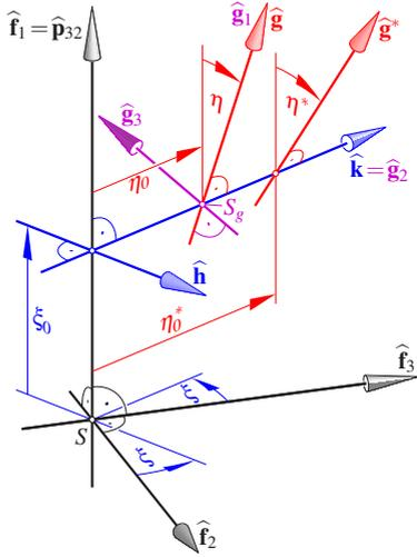
Figure 4: The triplet  $(\widehat{\mathbf{g}}_1, \widehat{\mathbf{g}}_2, \widehat{\mathbf{g}}_3)$  is the Frenet frame for the conjugate tooth flanks  $\Phi_2$  and  $\Phi_3$ . The corresponding Disteli axes  $\widehat{\mathbf{g}}^*$  are defined by the spatial Euler-Savary equation.
