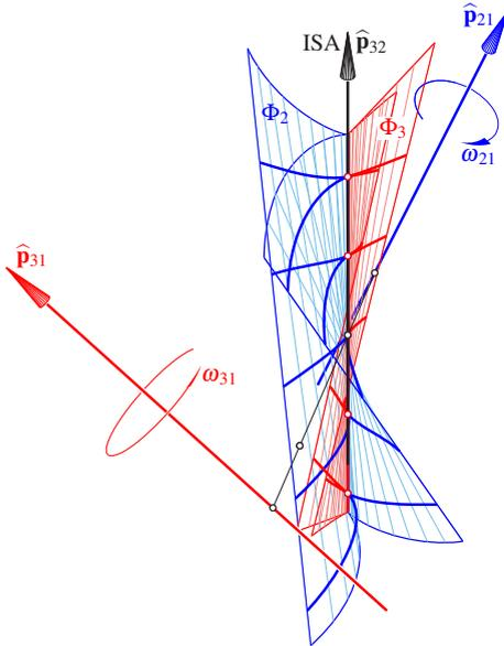
Figure 5: When the ISA coincides with the meshing line  $\widehat{\mathbf{g}}$ , the singular lines of the two flanks  $\Phi_2$ ,  $\Phi_3$  come together sharing the tangent plane at each point of  $\widehat{\mathbf{g}}$ ; but the flanks open toward opposite sides. The fat red and blue lines indicate sections orthogonal to the ISA.
