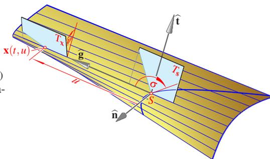
Figure 3: The distribution parameter  $\delta$  defines the tangent planes  $T_x$  along the generator  $\widehat{\mathbf{g}}$  by  $\tan \psi = -u/\delta$ . The angle  $\sigma$  between  $\widehat{\mathbf{g}}$  and the striction curve is called the *striction angle* or the *striction*.
