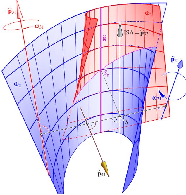
Figure 6: Two conjugate flanks  $\Phi_2$  and  $\Phi_3$  with  $G^2$ -contact at the common striction point  $S_g$ . The meshing line  $\hat{\mathbf{g}}$  is parallel to the ISA and a cylindric generator of  $\Phi_2$  and  $\Phi_3$ .
